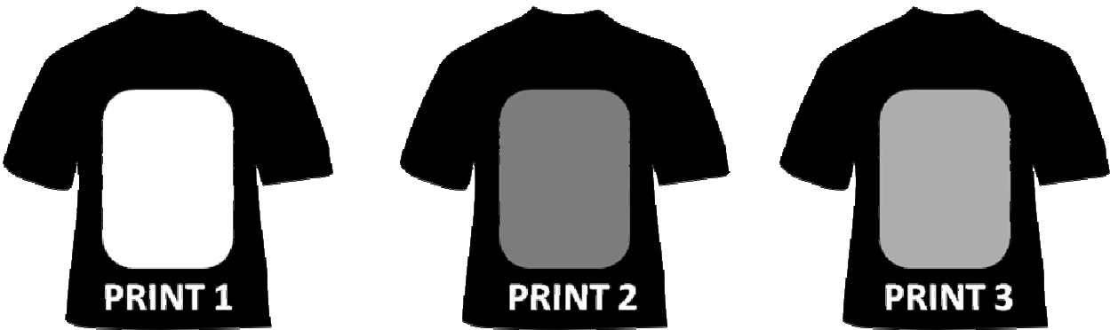
Figure 11: Inconsistent Print Platen to Platen (This can be observed in print or in residue on top of screen)
