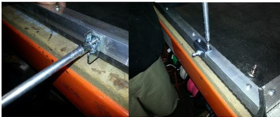
11. Replace the mounting brackets and latch hooks.
