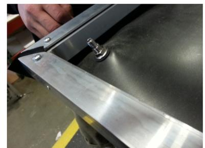
12. With the back of the lid facing you. (The back of the lid is the side that is opposite of the latch hooks) on the left corner closest to you about 2 inches away from each wall use a hole punch to put a small hole and put the valve stem into that hole facing up. (The order of the components for the valve stem goes as follows from bottom to top. Valve stem, rubber washer, neoprene blanket, rubber washer, metal washer, nut.)
