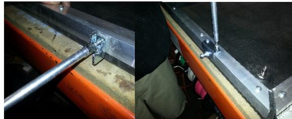
4. Remove the lid from the unit by using a phillips head screw driver to remove the screws from the hinge
