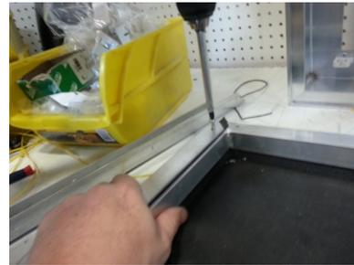
10. pull each support up onto the frame with the neoprene blanket in between the frame and the support. -Align the holes in the frame with the holes in the supports. since you will not be able to see the holes in the due to the neoprene being in the way, use one of the screws to poke into the support hole and feel out where the hole is. once you find the hole screw the support frame on. do this to each of the sides
