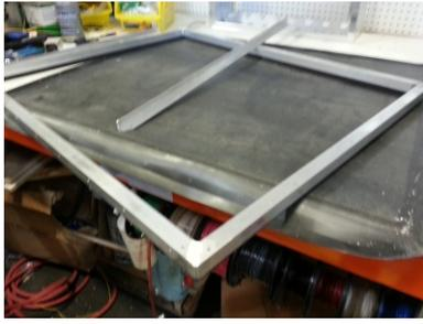
8. lay out the new neoprene blanket flat and place the square frame in the middle of the new blanket with the foam rubber facing down towards the neoprene
