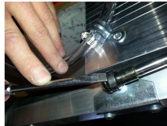
2. Remove Vacuum hose from the valve stem attached to the old neoprene blanket.
