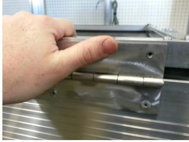
13. Place the lid on top on the Unit and reattach the lid to the hinge.
